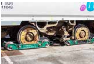
Day 11: It was the 2nd of April before the rescue succeeded. Never an ideal solution, 'Wheelskates' had nevertheless to be used to raise one of the damaged bogies above railhead level - so that the units could be moved to Ulverston Yard.
